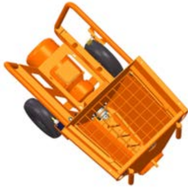
Figure 8: Material hopper assembly
