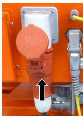
Figure 32: Connecting the power supply
