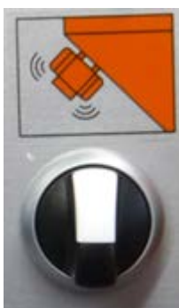
Figure 20: Selector switch - Vibrating unit
