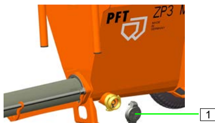
Figure 45: Opening the cleaning nozzles
