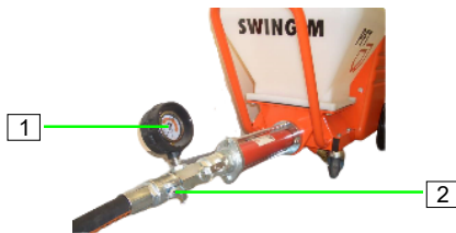
Figure 43: Disconnecting the water hose
