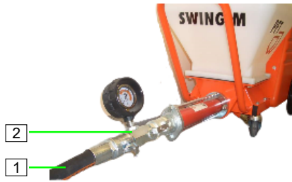
Figure 21: Connecting the mortar hose
