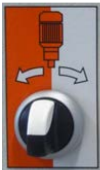
Figure 14: Pump motor selector switch
