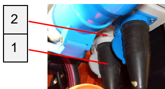
Fig. 59: Connect vibrating unit
