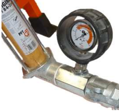
Fig. 29: Mortar pressure gauge
