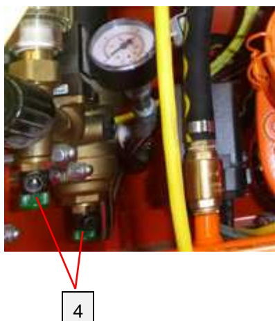
Fig. 107: Open the drain tap
