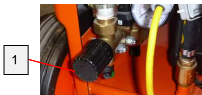
Fig. 114: Pressure reducing valve
