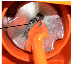
Fig. 100: Drive dog position
