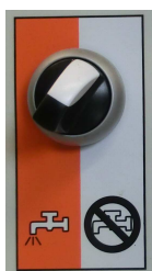
Fig. 18: Selector switch Water
