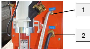
Fig. 15: Connection Water and Air
